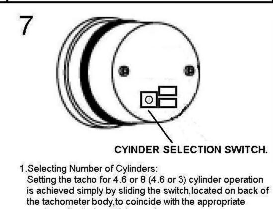
the tachometer body,to coincide with the appropriate number of cylinders of the engine.
