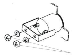
Do not over tighten bolts when installing U bracket. Doing so will cause damage to movement inside.
