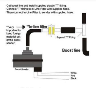
Black- Ground Red- 12v Accessory Power White- Green wire from gauge Do not over tighten bolts when installing II bracket. Doing so will
