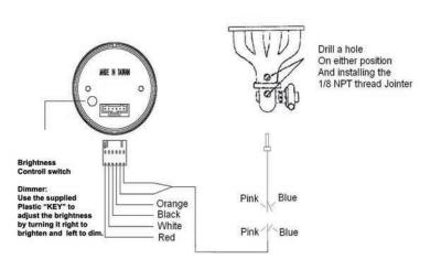
You will need to drill and tap a 1/8th NPT fitting for the probe to go into. We recommend a professional to tap this. Try to avoid shavings from going into the manifold or exhaust.
